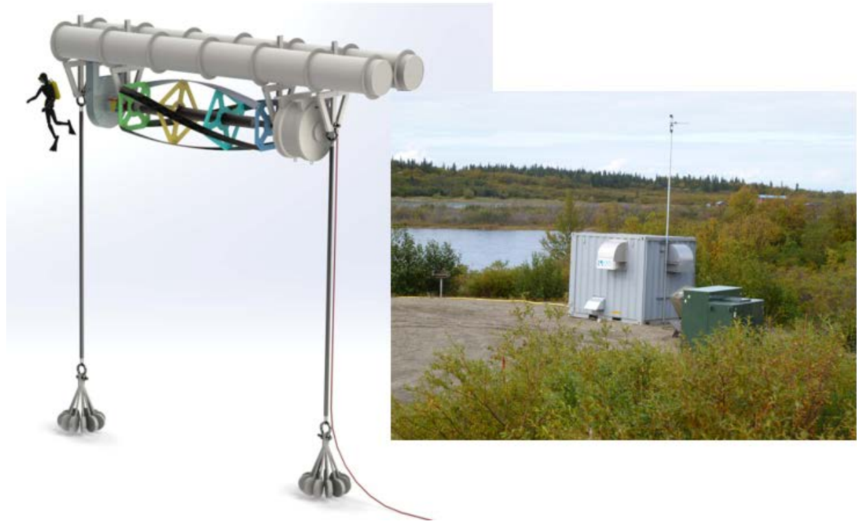
Figure 3. Potential test system for the deployment and retrieval subsystem test. Diver is included only for size reference, as it is not anticipated that a diver will be required except for near shore connections to the anchors. Anchors will be gravity anchors of undetermined design.
