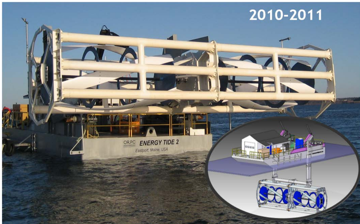
Figure 1. The turbine performance testing of the Advanced TidGen® turbines will be performed in a barge tow test similar to several tests performed by ORPC on earlier turbine designs.
